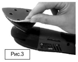
The sanding plate (8) is equipped with velcro for fast and easy changing of the sanding cloth (11), which is also equipped with velcro.
